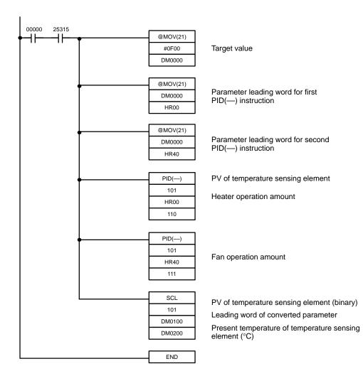
**Note** When using PID(—) or SCL(—), make the data settings in advance with a Peripheral Device such as the Programming Console or LSS.
